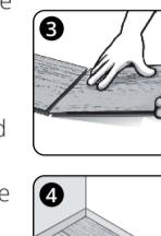
**3.** Connect the short sides when laying the first row (Figure 3). Lay the keys of every new panel precisely over the groove of the previous panel on the short side and hit them from the top with the rubber panel. This is particularly important for a good connection.
