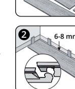
**2.** The laying should be started in a corner (left side) with the groove facing the wall. Observe an edge distance of 6-8 mm to compensate the expansion of the ISOCORE floorboards in case of temperature changes (Figure 2).
